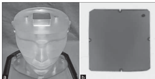
Figure 6: (a) 40 mm × 40 mm Gafchromic EBT3 film placed in the phantom for irradiation and (b) the exposed film with fiducial marks on the films
