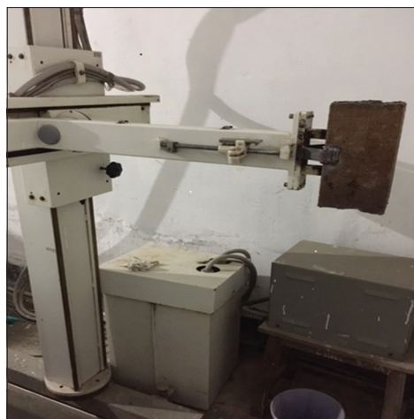
Figure 2: L Arm with new counterweight
