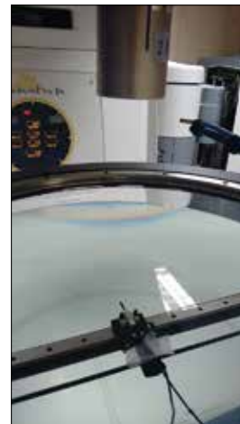
Figure 1: Experimental setup for measurement of total scatter factor.
