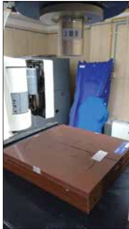
Figure 2: Experimental setup for calibration of plastic scintillator detector (buildup is removed for clear view of detector).
