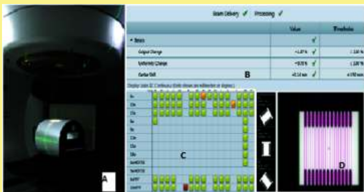
Fig. (A) IsoCal Phantom mounted on True Beam Couch, (B) Tabulated result of Dosimetric Check, (C) MPC evaluation window, (D) Open field with comb-like MLC pattern for treatment isocenter definition.
